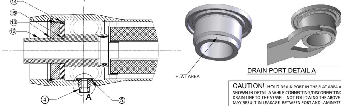
CAUTION!: HOLD DRAIN PORT IN THE FLAT AREA AS SHOWN IN DETAIL A WHILE CONNECTING/DISCONNECTING DRAIN LINE TO THE VESSEL. NOT FOLLOWING THE ABOVE MAY RESULT IN LEAKAGE BETWEEN PORT AND LAMINATE
